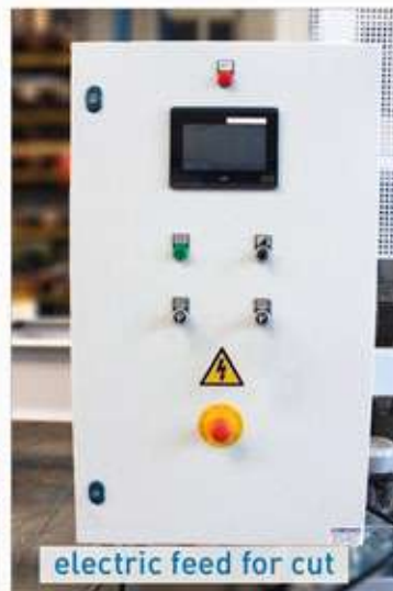
touchscreen with digital readout, 8 lengths can be memorized (optionally repositionable)
